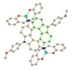
Combining photoactive bridging ligands with magnetic metal ions: Reaction of a fluorescent aryl-substituted carbazole ligand with copper(II) and zinc(II) ions results in the formation of metallacycles of the general formula  $[M_2L_2]$ . The fluorescent bridging ligand mediates antiferromagnetic exchange coupling between the copper centers.
